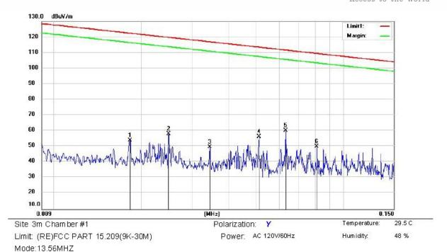
Correct Antenna Reading Measure-Table Limit Over No. Mk. Freq. Level Factor ment Height Degree MHz dBu∀ dΒ dBu∀/m dBuV/m dΒ Detector cm degree Comment 20.59 0.0182 33.36 53.95 122.39 -68.44 1 peak 0.0247 20.59 2 37.57 58.16 119.74 -61.58 peak 0.0343 29.21 3 20.63 49.84 116.89 -67.05 peak 4 0.0510 35.66 20.79 56.45 113.44 -56.99 peak 5 0.0631 39.47 20.72 60.19 111.59 -51.40 peak
