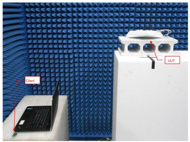
Note: The UUT main beam of the antenna is directly toward the radar emitter during testing.
