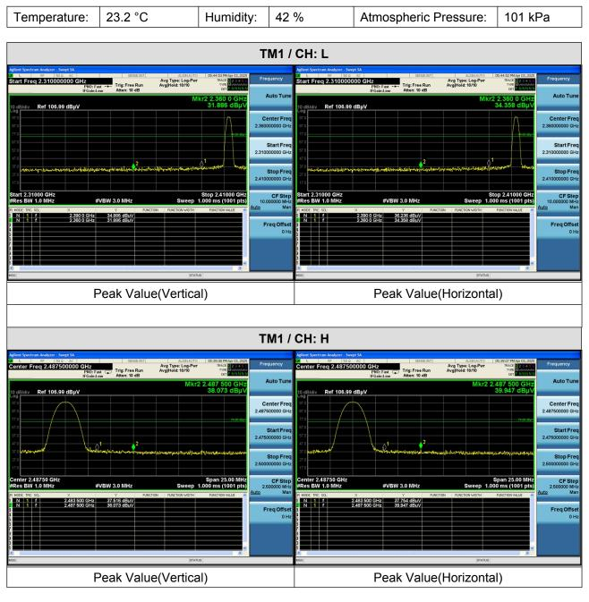
Remark: When the PK measure result value is less than the AVG limit value, the AV measure result values test not applicable.
