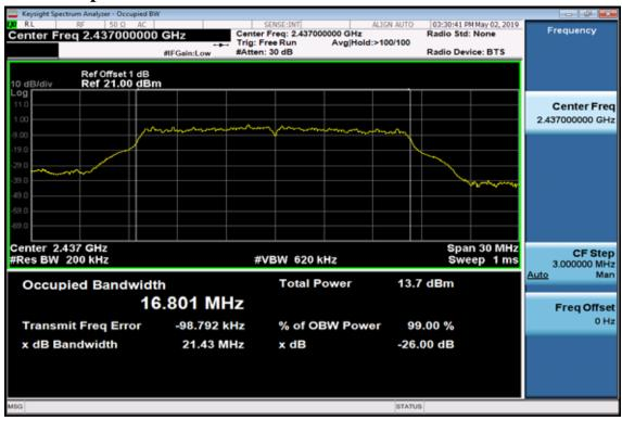
99% Occupied Bandwidth Test Data CH-High
