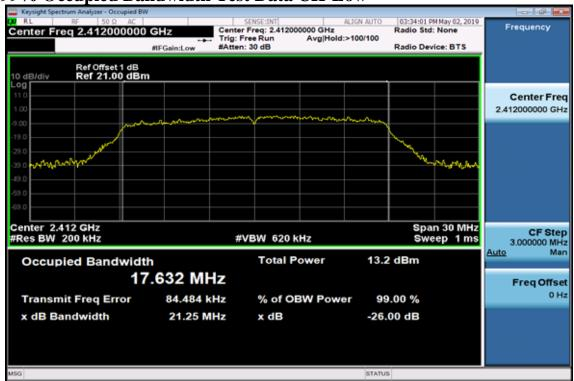
99% Occupied Bandwidth Test Data CH-Mid
