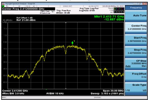
**Power Spectral Density Test Plot (CH-Mid)**
