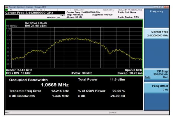
99% Occupied Bandwidth Test Data CH-High
