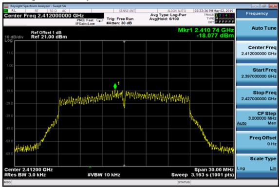
**Power Spectral Density Test Plot (CH-Mid)**
