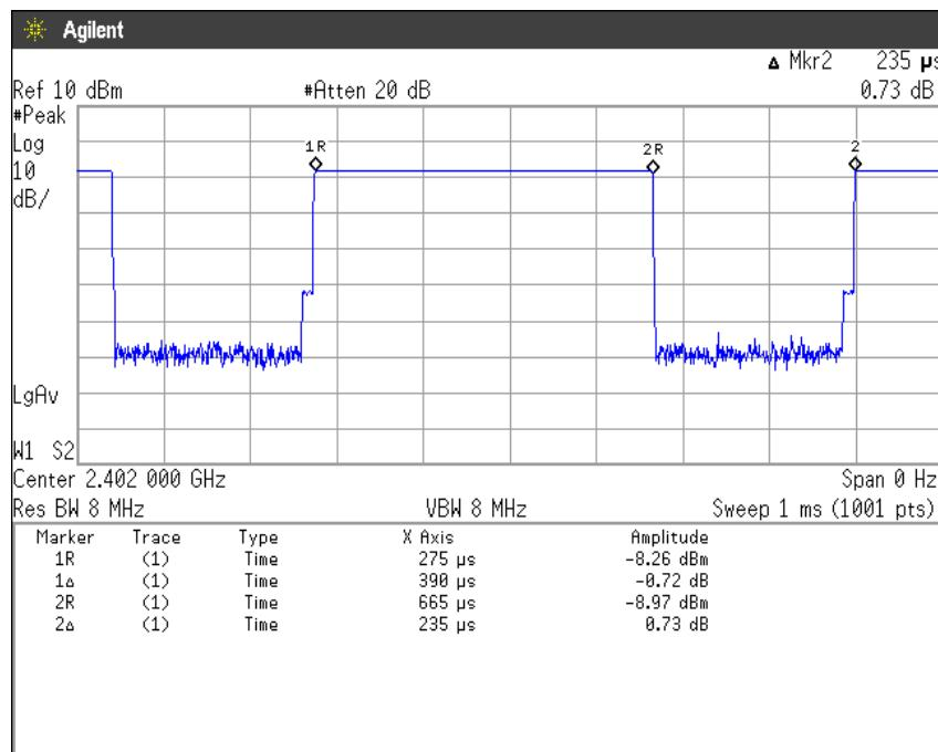
$$\text{Duty Cycle} = \text{Ton} / (\text{Ton} + \text{Toff}) = 390[\mu\text{s}] / (390[\mu\text{s}] + 235[\mu\text{s}]) = 62.4[\%]$$
