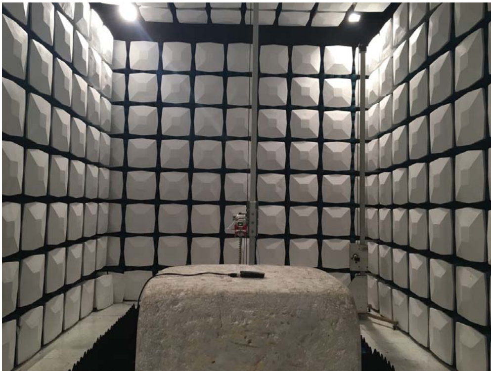
Description: Radiated Emission Test Setup for 1~18GHz
