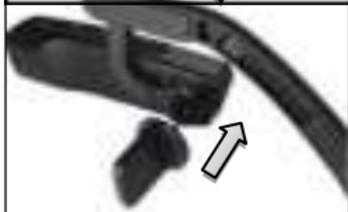
Step ❸ : Adjust the correct angle of the camcorder and use the small spanner to tighten the set screw.
