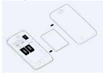
Finally insert the battery and replace the rear cover of the mobile phone.
