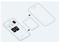
Finally insert the battery and the rear cover of the mobile phone.
