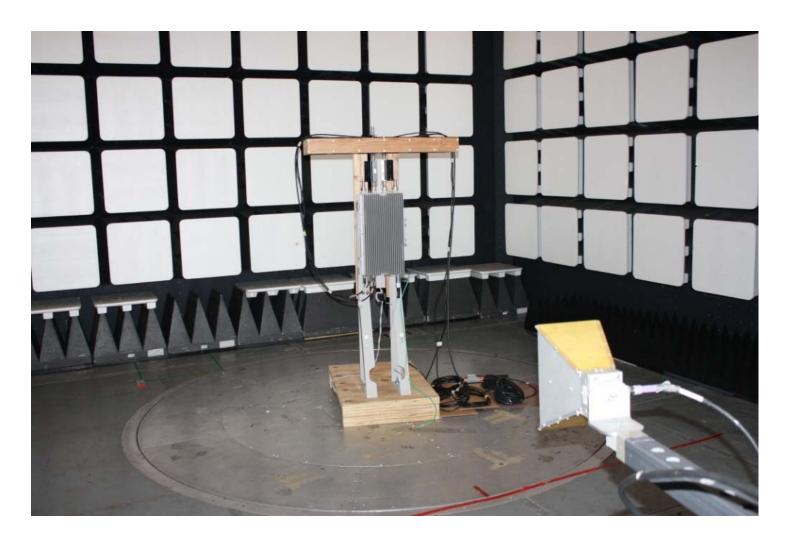
**TEST:** Measurement of Radiated Spurious Emissions
