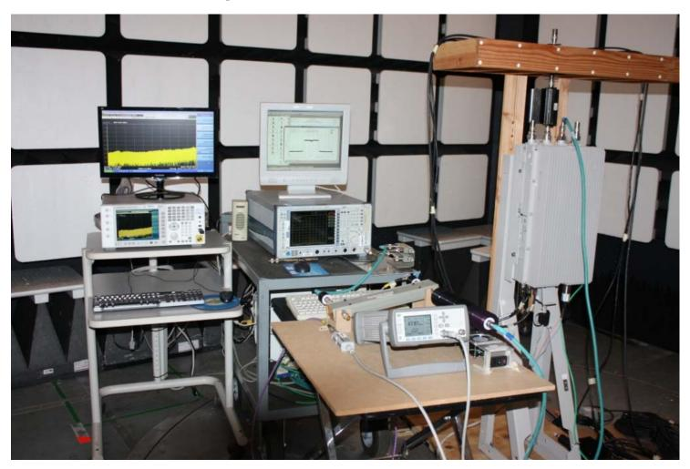
**TEST:** Measurement of Radiated Spurious Emissions
