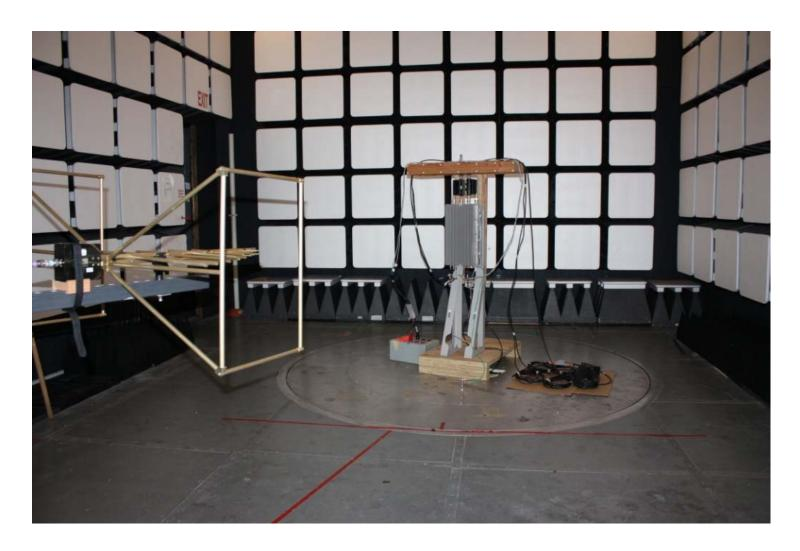
**TEST:** Measurement of Radiated Spurious Emissions
