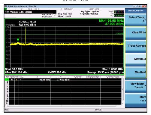
Conduct Spurious Emission (worst) @ 161.610MHz With 12.5 KHz Channel Separation-1W 1GHz-12.75GHz
