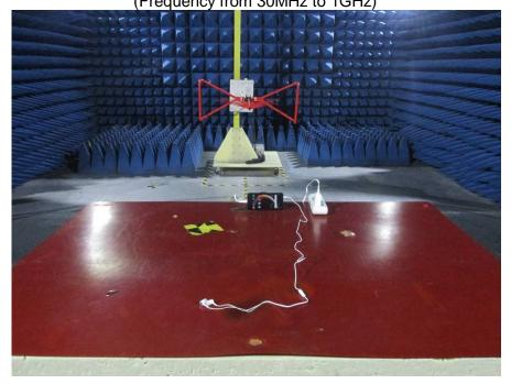
RADIATED EMISSION TEST (Frequency above 1GHz)
