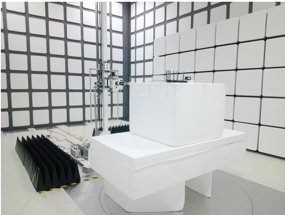
Description: Radiated Emission Test Setup for 18GHz~40GHz
