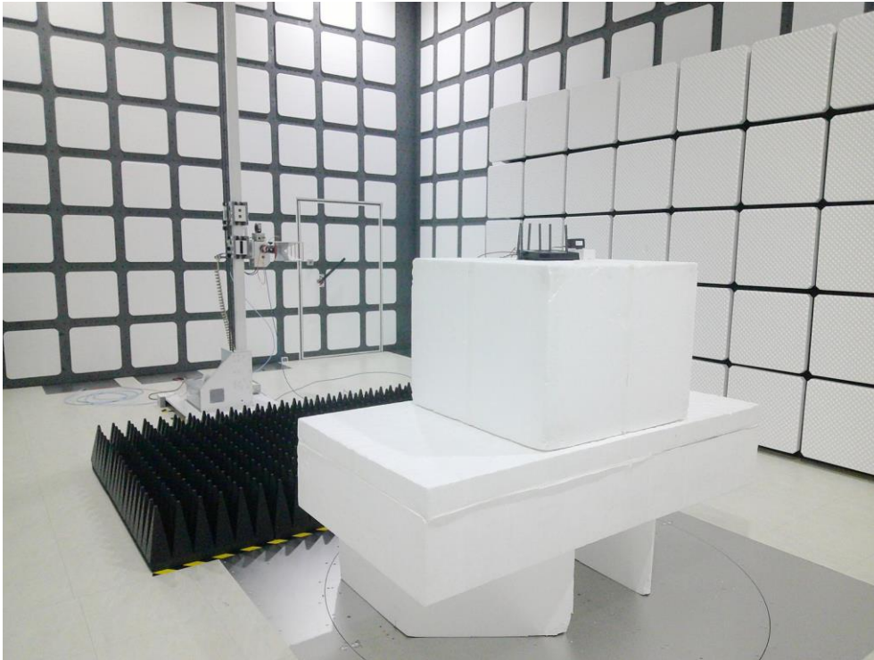
Description: Radiated Emission Test Setup for 18GHz~40GHz
