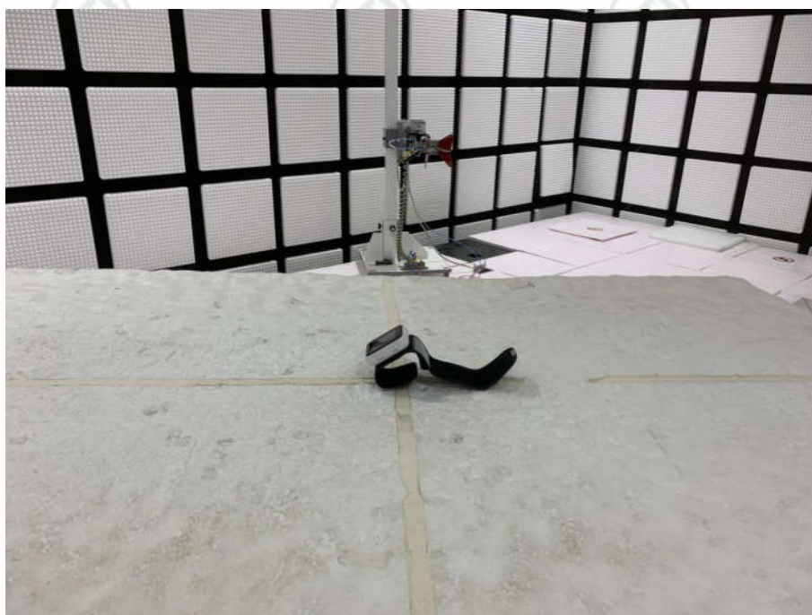
Radiated spurious emission Test Setup-2(Above 1GHz)
