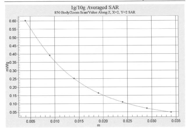
Fig. 26 Z-Scan at power reference point (Flat Phantom 850MHz CH251 with the display of the handset towards the ground)
