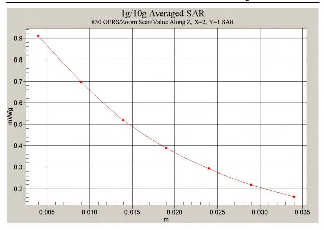
Fig. 40 Z-Scan at power reference point (Flat Phantom 850MHz CH190 GPRS with the display of the handset towards the ground)
