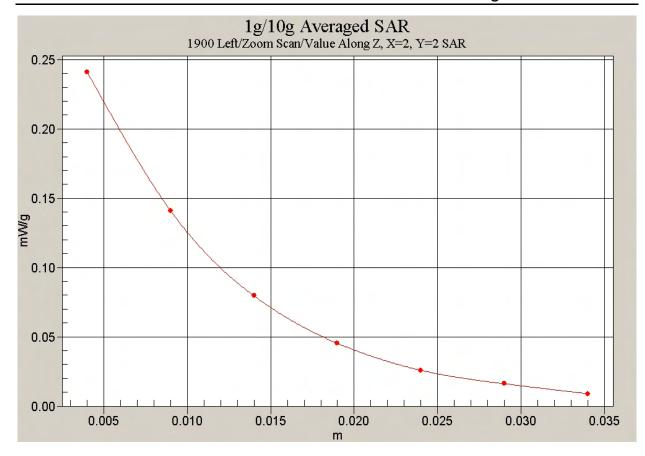
Fig. 52 Z-Scan at power reference point (Left Hand Touch Cheek 1900MHz CH661)
