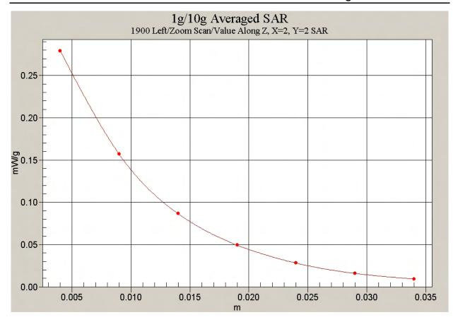
Fig. 58 Z-Scan at power reference point (Left Hand Tilt 15° 1900MHz CH661)
