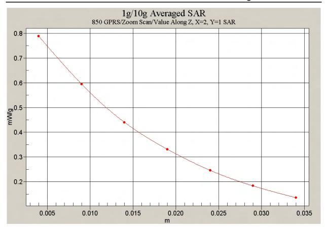
Fig. 38 Z-Scan at power reference point (Flat Phantom 850MHz CH251 GPRS with the display of the handset towards the ground)
