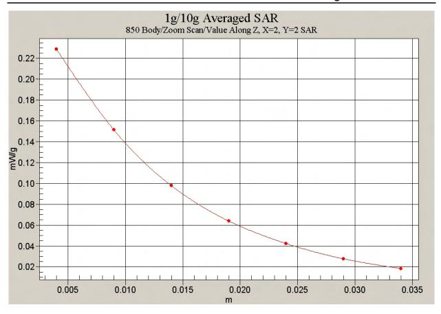
Fig. 34 Z-Scan at power reference point (Flat Phantom 850MHz CH190 with the display of the handset towards the phantom)
