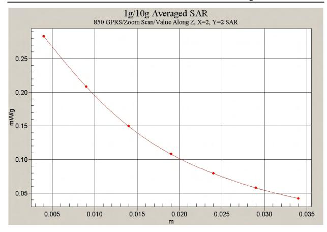
Fig. 44 Z-Scan at power reference point (Flat Phantom 850MHz CH251 GPRS with the display of the handset towards the phantom)
