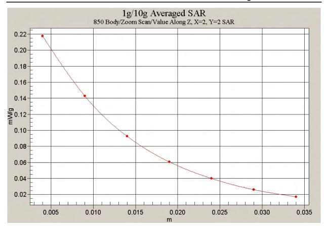
Fig. 32 Z-Scan at power reference point (Flat Phantom 850MHz CH251 with the display of the handset towards the phantom)
