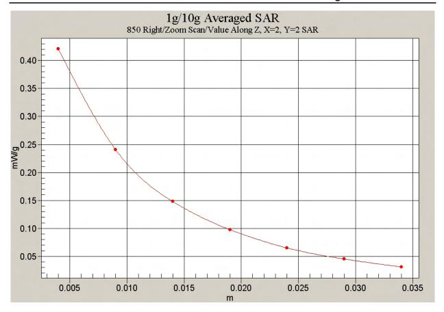
Fig. 20 Z-Scan at power reference point (Right Hand Tilt 15° 850MHz CH251)
