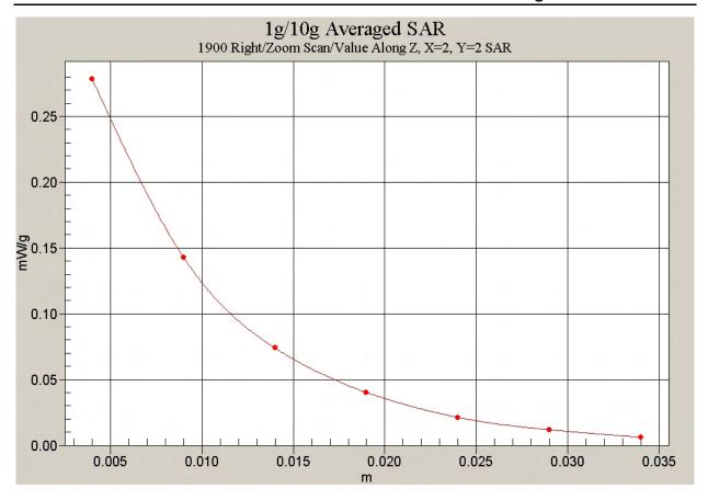
Fig. 62 Z-Scan at power reference point (Right Hand Touch Cheek 1900MHz CH810)
