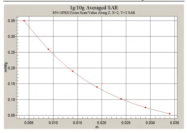
Fig. 46 Z-Scan at power reference point (Flat Phantom 850MHz CH190 GPRS with the display of the handset towards the phantom)
