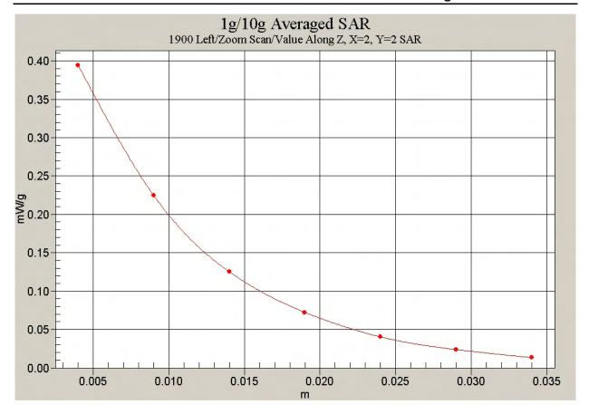
Fig.60 Z-Scan at power reference point (Left Hand Tilt 15° 1900MHz CH512)
