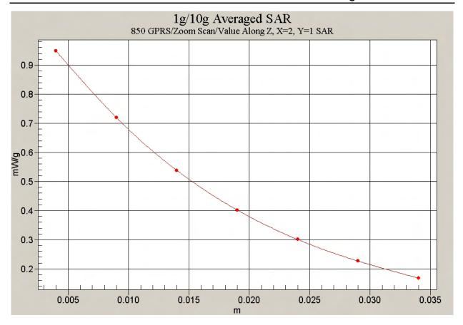
Fig. 42 Z-Scan at power reference point (Flat Phantom 850MHz CH128 GPRS with the display of the handset towards the ground)
