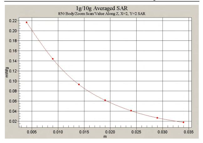
Fig. 36 Z-Scan at power reference point (Flat Phantom 850MHz CH128 with the display of the handset towards the phantom)
