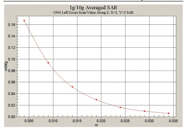
Fig. 56 Z-Scan at power reference point (Left Hand Tilt 15° 1900MHz CH810)
