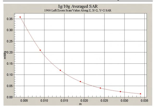
Fig. 54 Z-Scan at power reference point (Left Hand Touch Cheek 1900MHz CH512)
