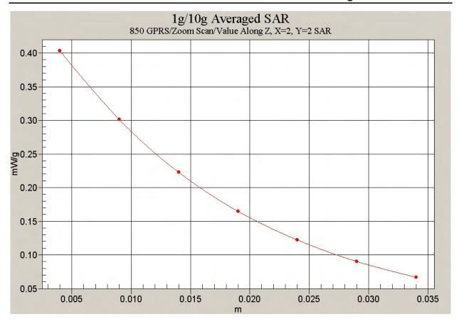
Fig. 48 Z-Scan at power reference point (Flat Phantom 850MHz CH128 GPRS with the display of the handset towards the phantom)
