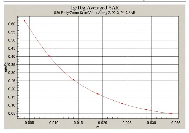
Fig. 30 Z-Scan at power reference point (Flat Phantom 850MHz CH128 with the display of the handset towards the ground)
