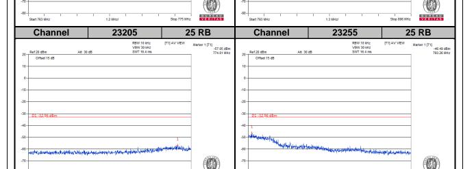
For the 763 - 775 MHz and 793 - 805 MHz band, the FCC limit is 65+10log(P[watt]) in a 6.25 kHz bandwidth. Since it was not possible to set the resolution bandwidth to 6.25 kHz with the available equipment, a bandwidth of 10 kHz was used instead to show compliance. By using a 10 kHz bandwidth on the spectrum analyzer.
