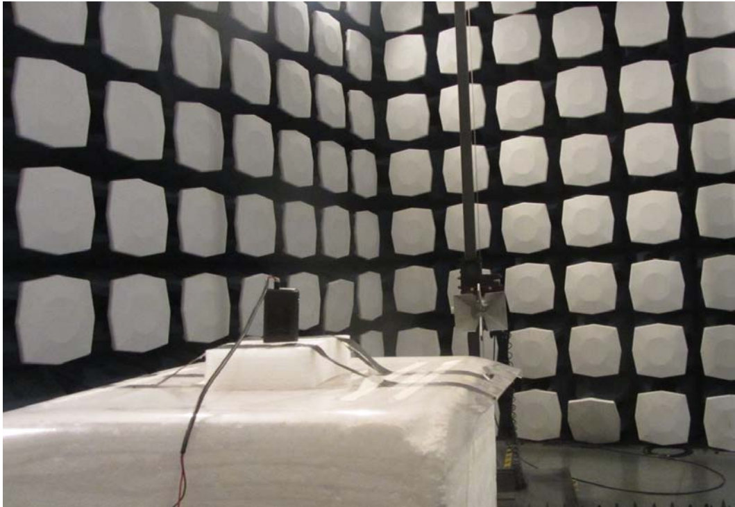
Picture 2: Radiated Spurious Emissions Test setup
