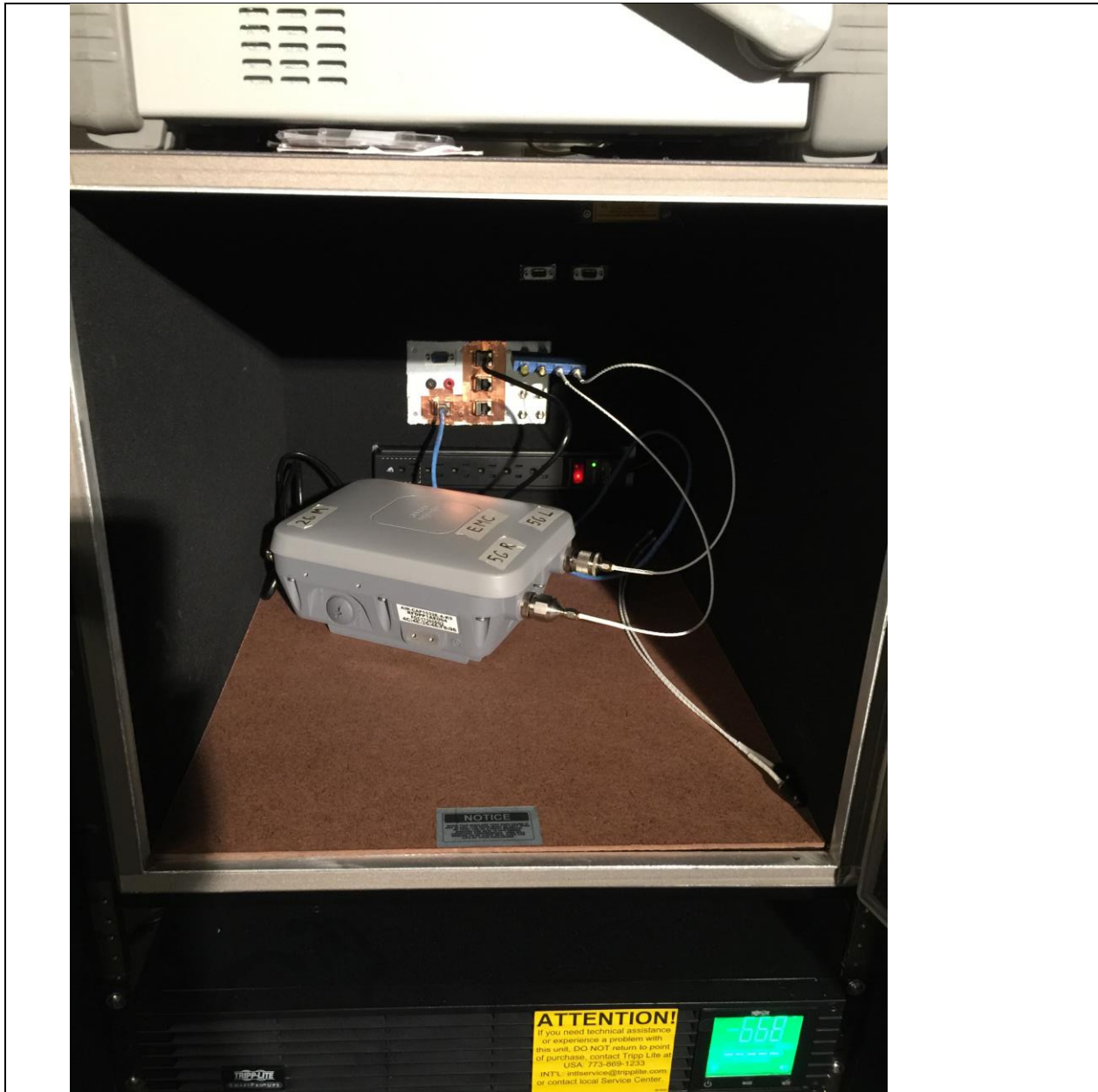
Title: AIR-CAP1532E-B-K9 Conducted Test Setup
