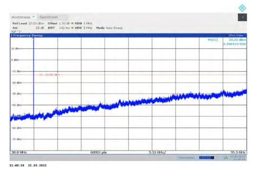
n77H NOTE: peak above the limit line is the carrier frequency.
