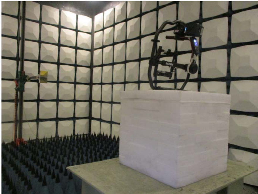
Radiated Emission View (Above 1GHz)
