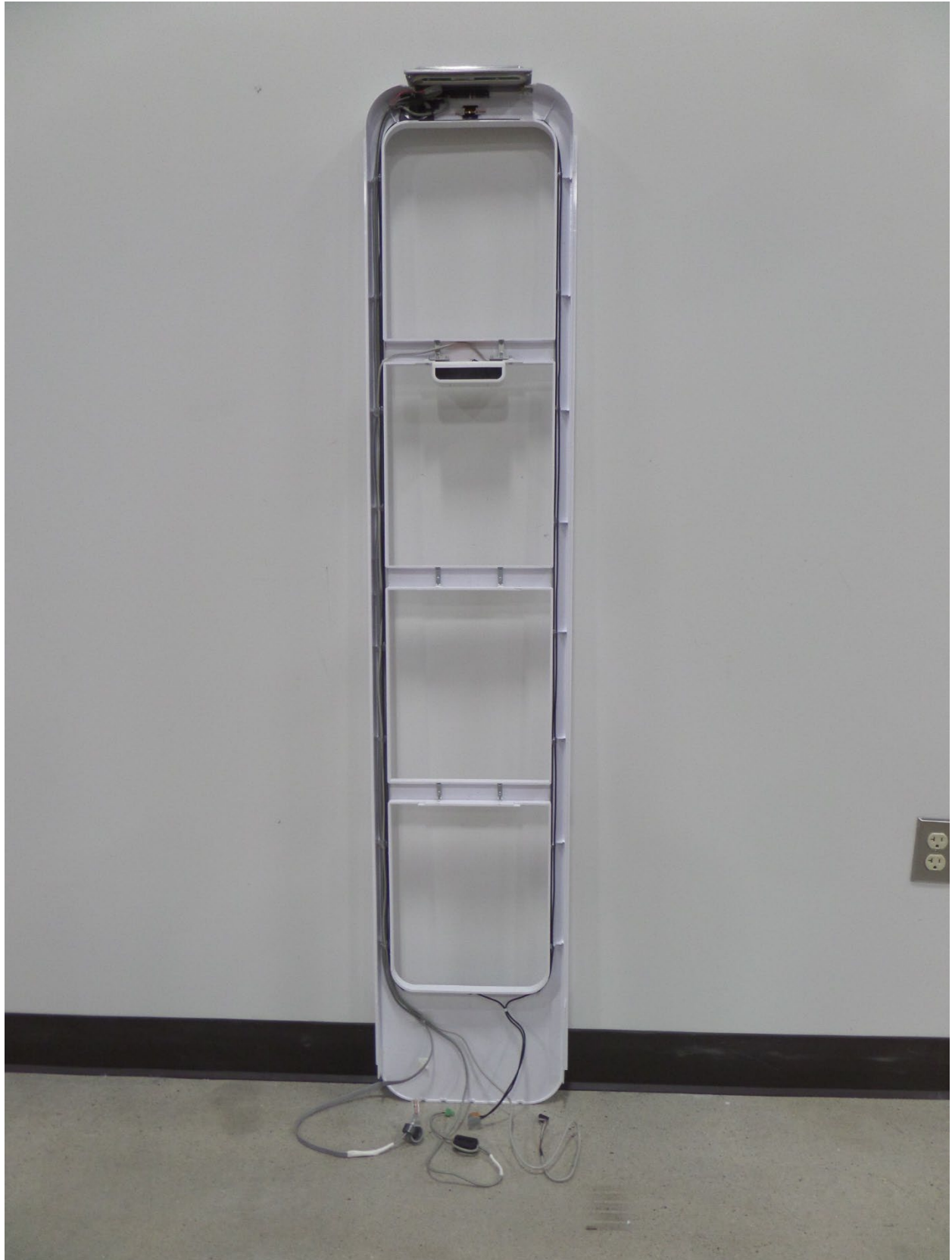
Figure 3: NP22 PRI/PAB/SAB RF ANT FRAME FRONT SIDE
