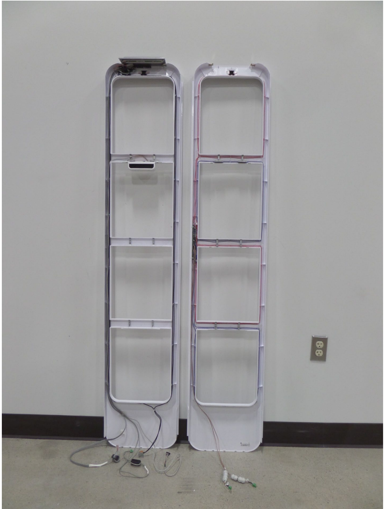
Figure 1: NP22 PRI/PAB/SAB RF ANT FRAME TWO HALVES
