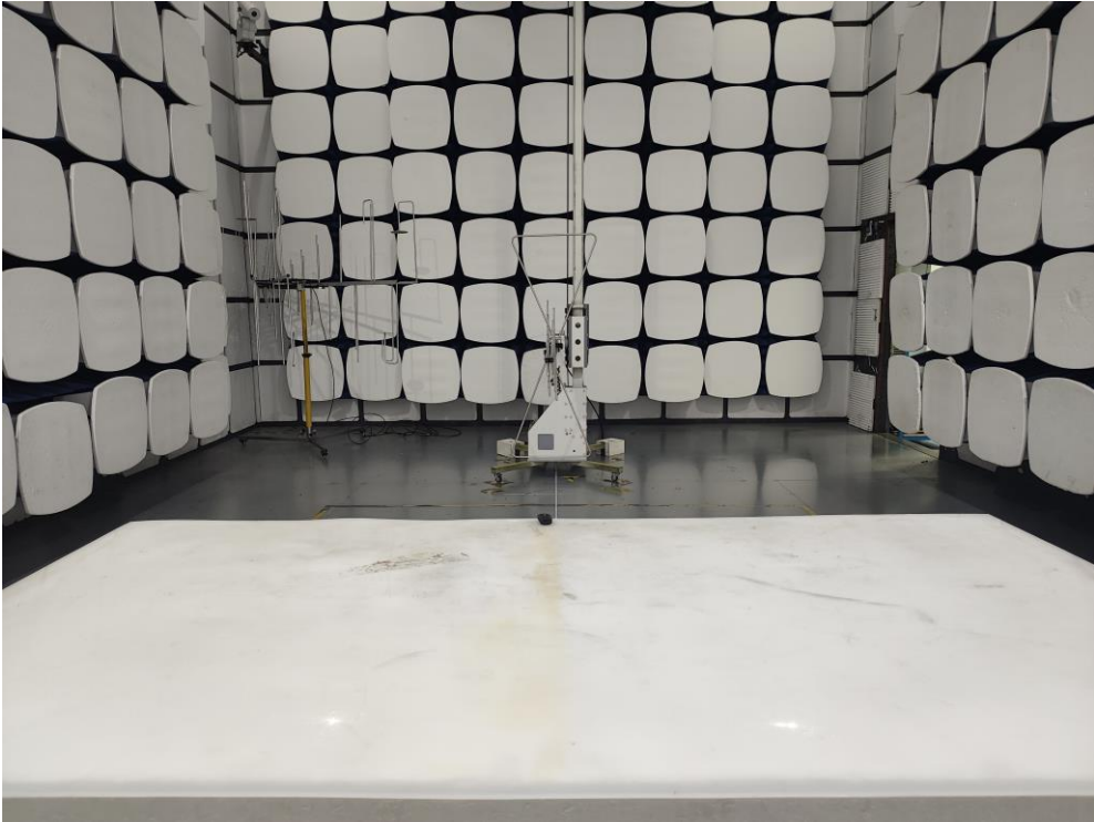
Photo of Radiated Emission test
