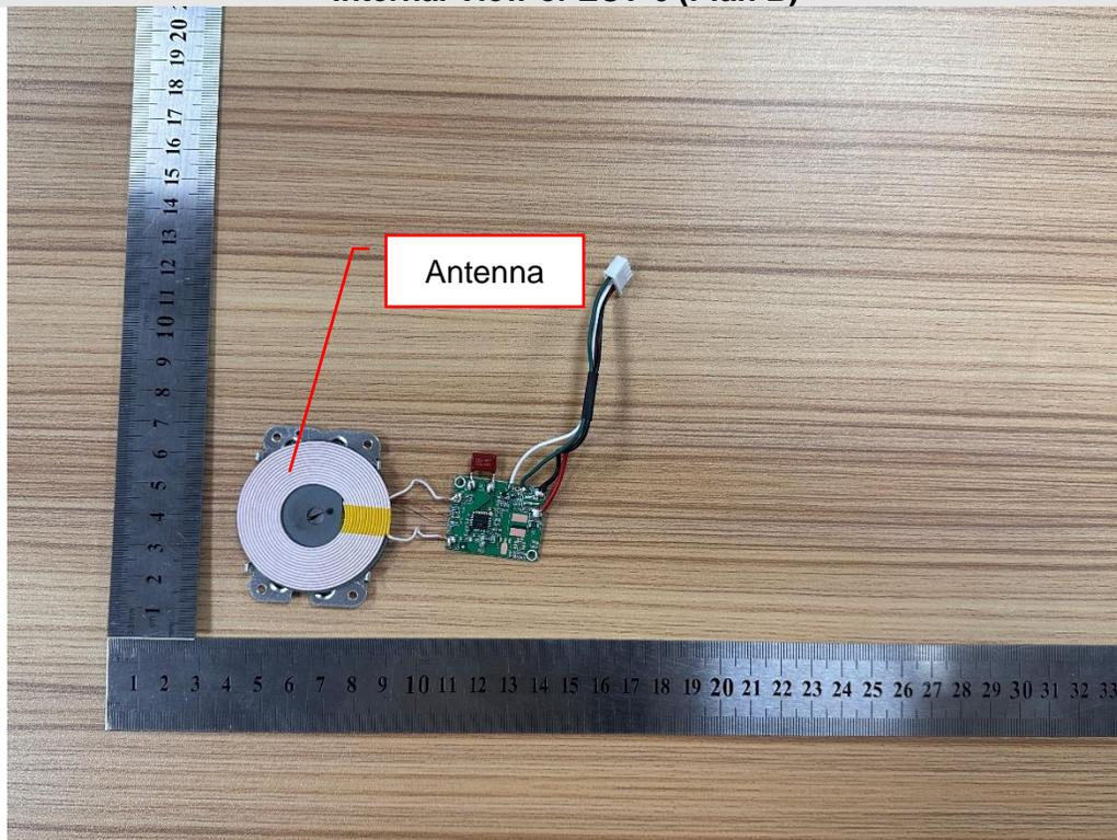
**Internal View of EUT-7 (Plan B)**
