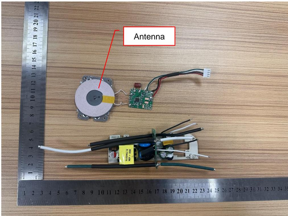
**Internal View of EUT-13 (Plan A)**
