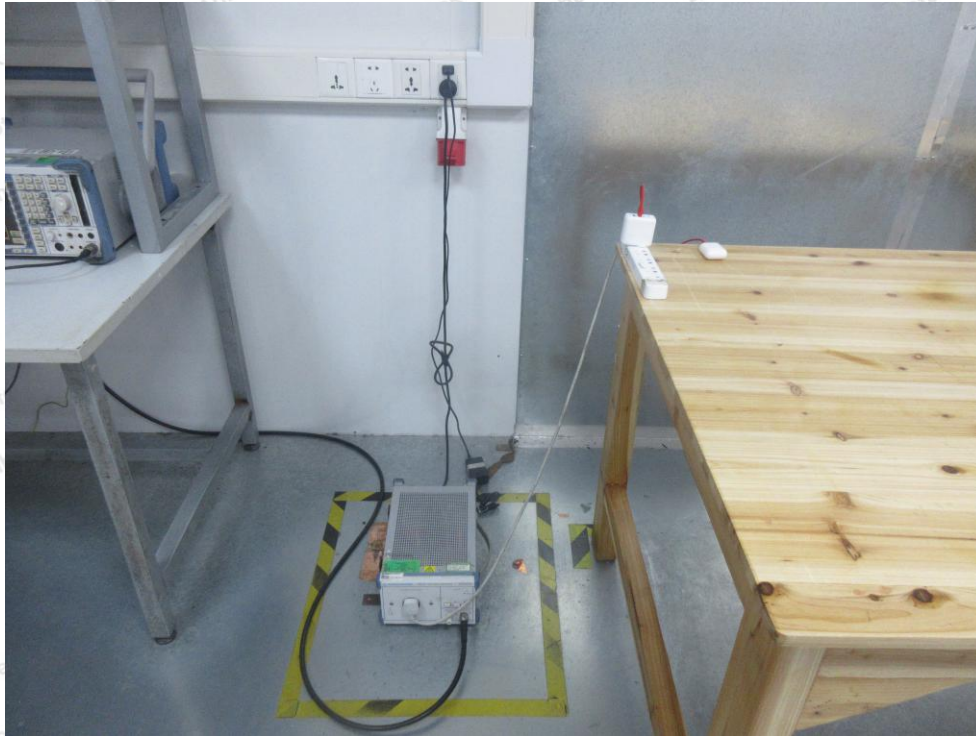
Photo of Power Line Conducted Emission Test
