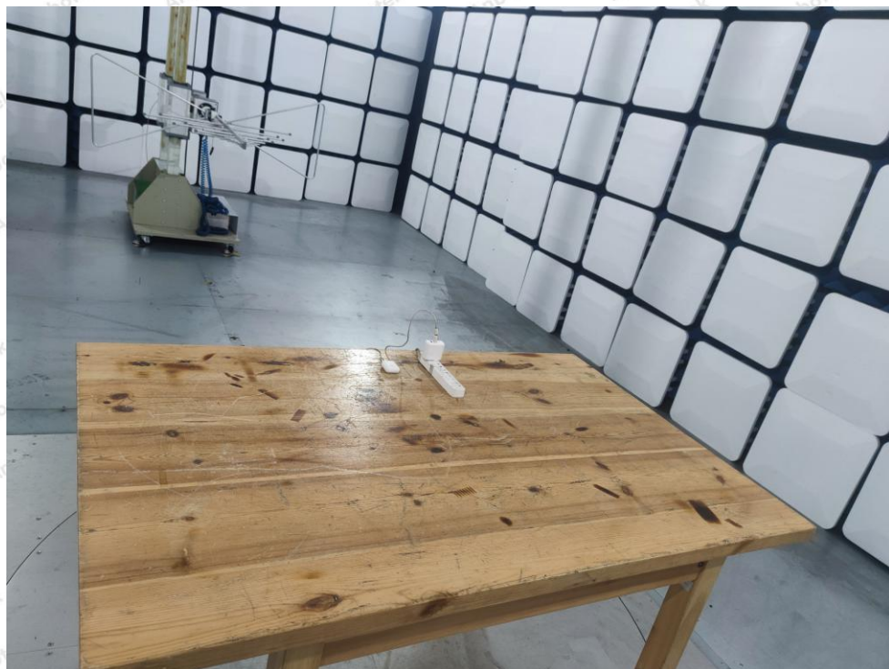
Photo of Radiation Emission Test
