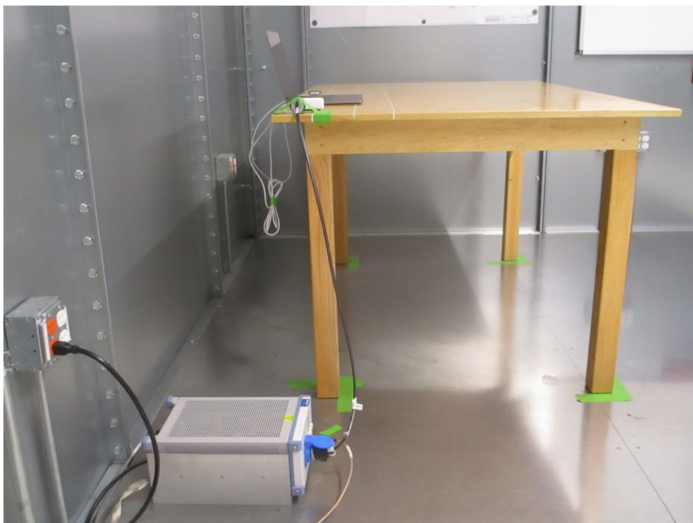
Figure 4: AC Line Conducted Emissions (Side View)
