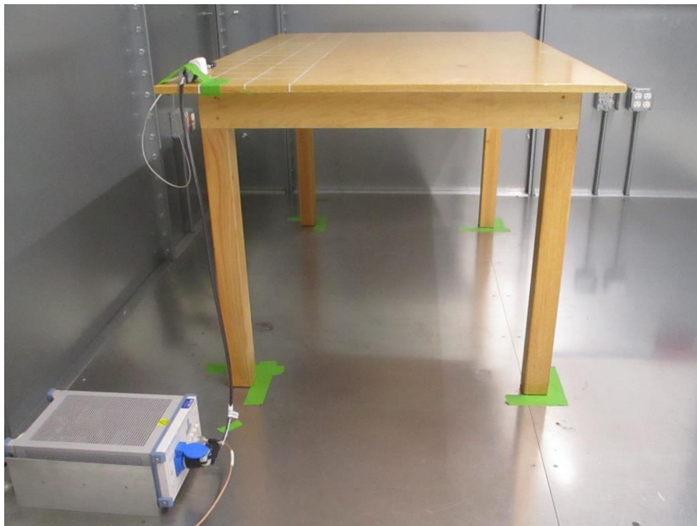
Figure 2: AC Line Conducted Emissions (Side View)
