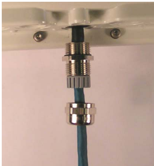
Step 2: Insert the RJ45 connector making sure that the locking tab snaps home
