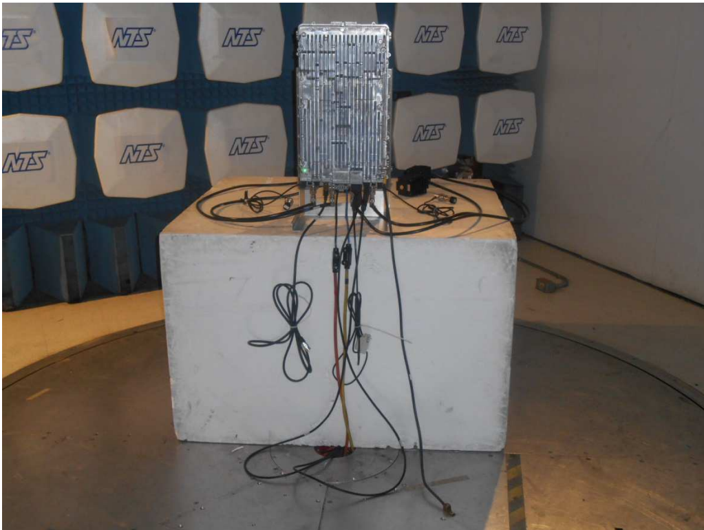
Radiated Emissions Setup - Front
