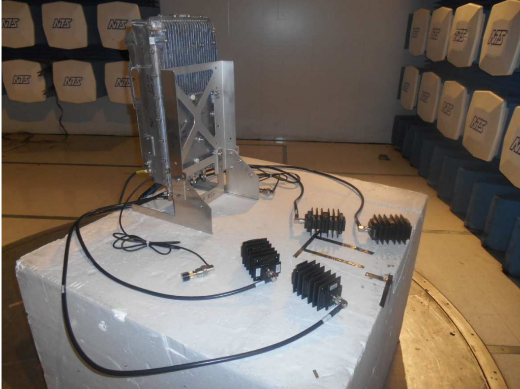
Radiated Emissions Setup – Rear
