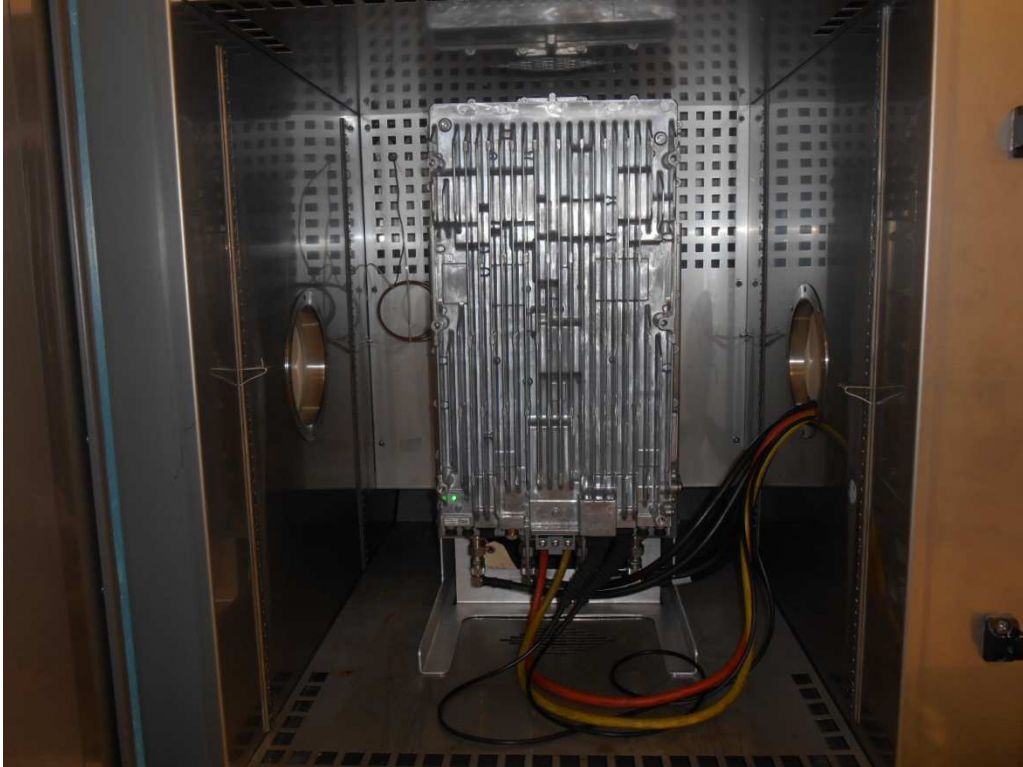
Frequency Stability Setup
