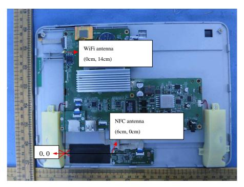
The power densities of up to 2 antennas located within a 90 cm<sup>2</sup> region at 1cm intervals are estimated first. Then the power densities computed for each antenna are summed.
