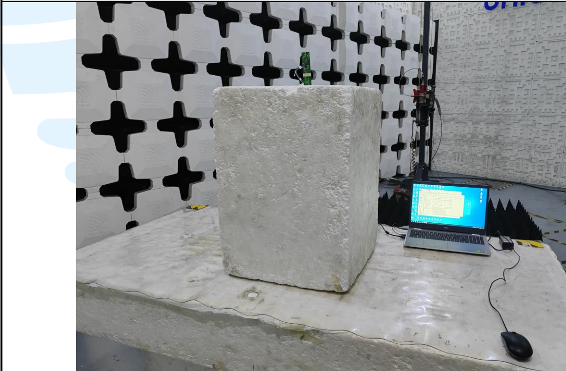
Radiated emission Test Setup (Above 1 GHz)
