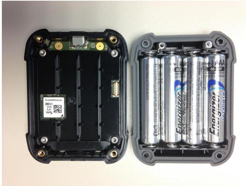
Trace PCBA / Battery Separator Installed Over PCBA in Top Enclosure (Left)
