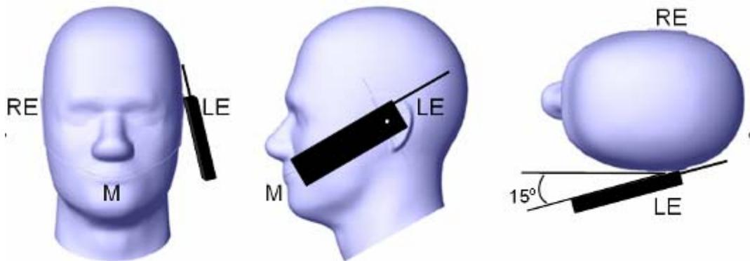
**Test positions for body-worn and other configurations**
