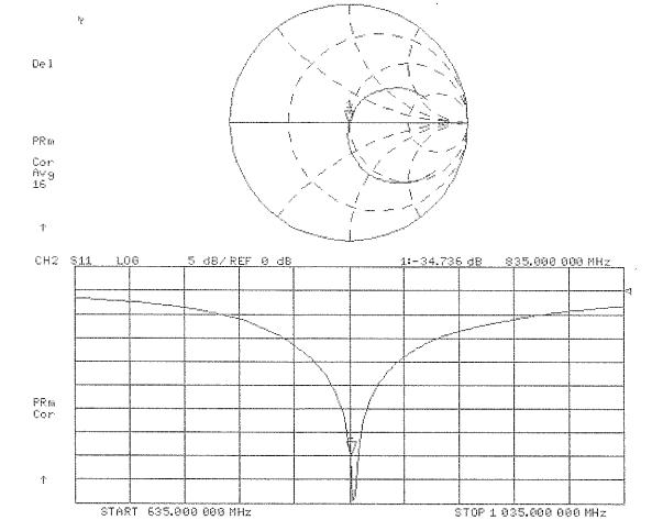
Validation Dipole D835V2 SN455, d = 15 mm
