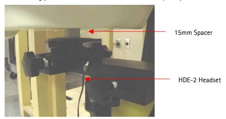
Note: the 15mm spacer was removed before the SAR measurement.
