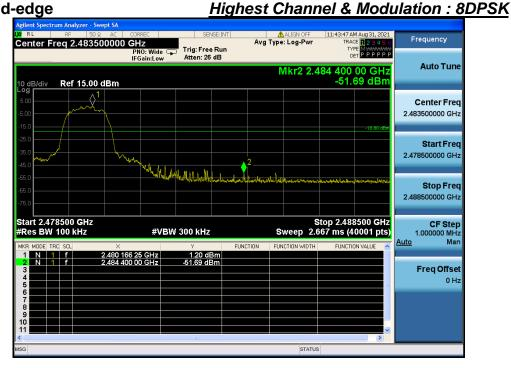
High Band-edge <u>Hopping mode & Modulation : 8DPSK</u>
