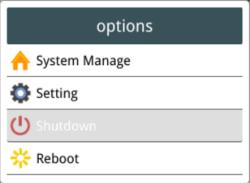
Select "Shutdown" menu using "▲", "▼" arrow keys or "2", "8" and then press <OK> key.
