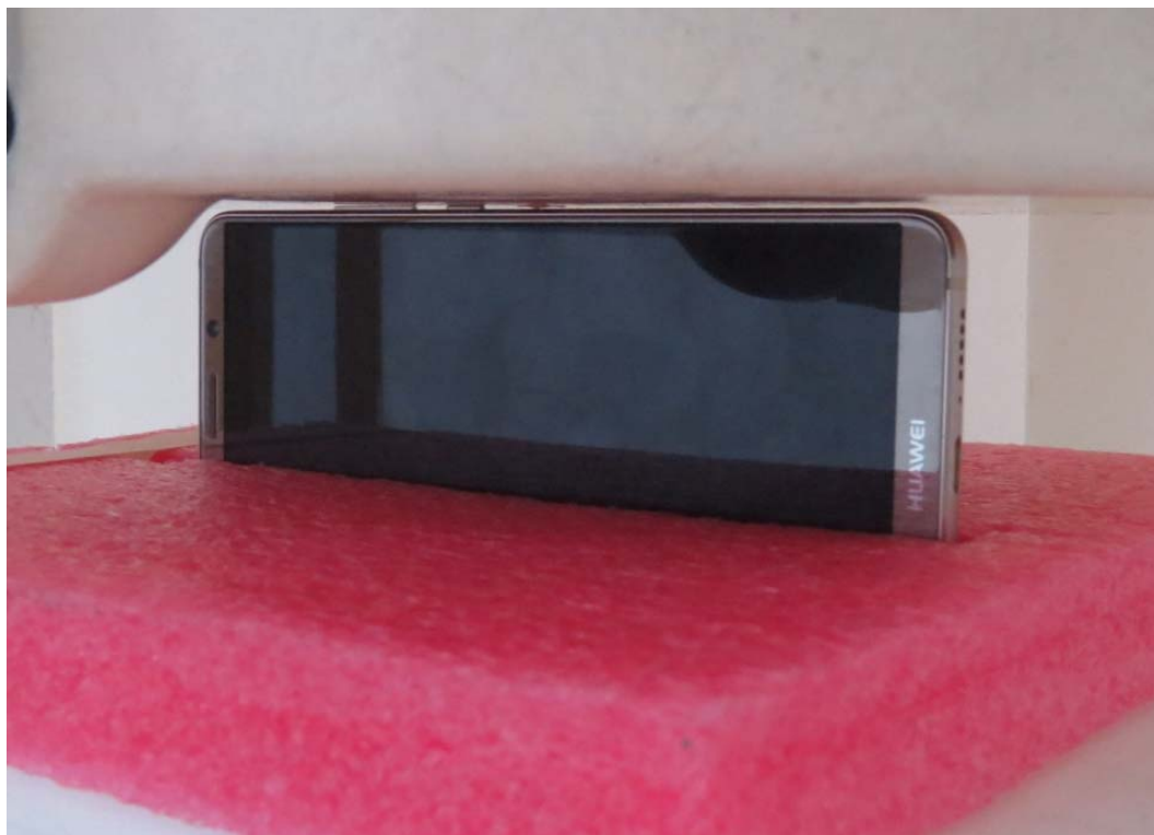
Picture 40: Right Side, the distance from handset to the bottom of the Phantom is 0mm
