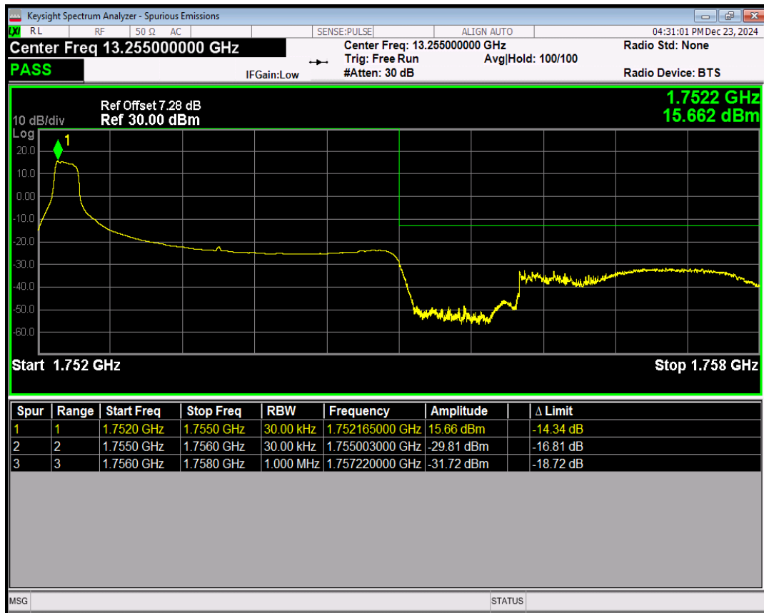
Band4 16QAM BW=3MHz Channel=20385 RB Size=1 Position=#Max
