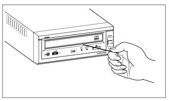
After manually ejecting a disc, you must turn off the power supplied to the CRW4416SX, then turn it on before continuing.
