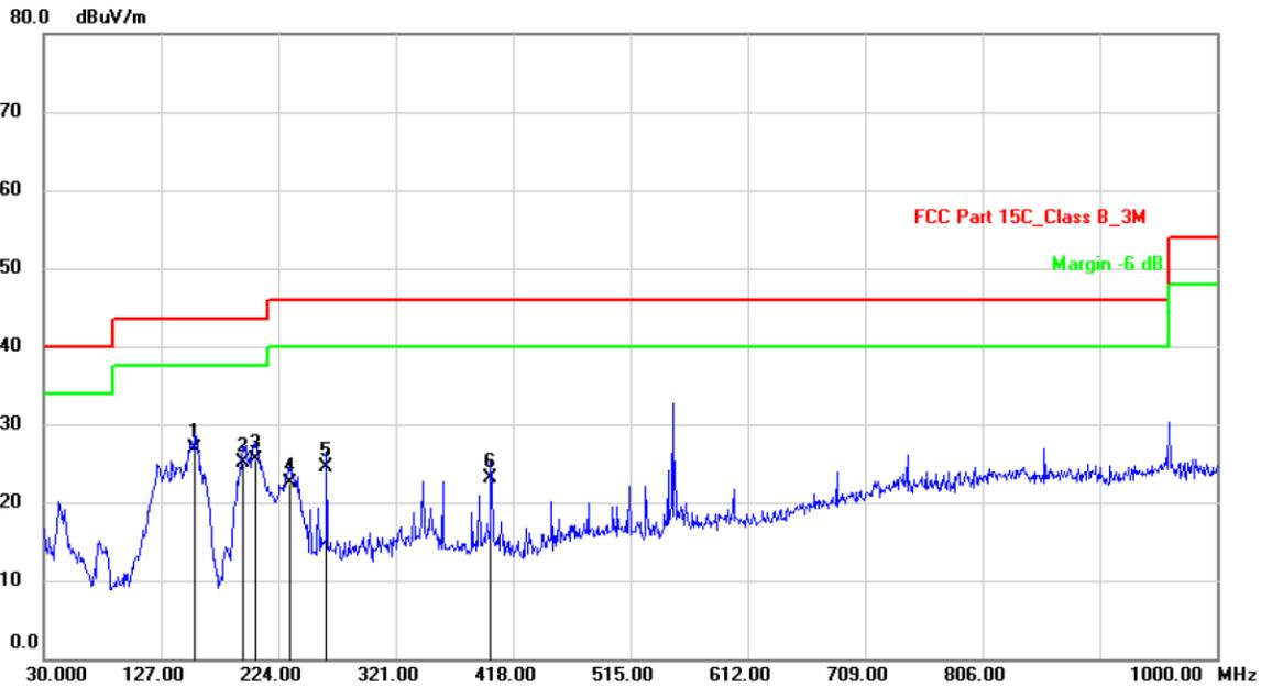
Site: 3m Chamber                      Polarization: **Vertical**                      Temperature: 26
