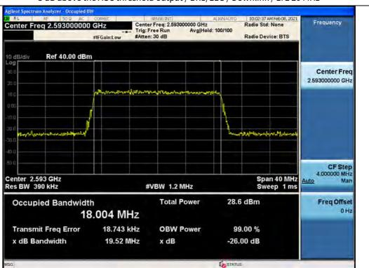
3 dB above the AGC threshold output / BRS/EBS / Downlink / LTE 20 MHz
