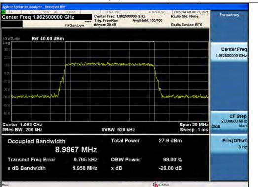
3 dB above the AGC threshold output / Broadband PCS / Downlink / LTE 10 MHz
