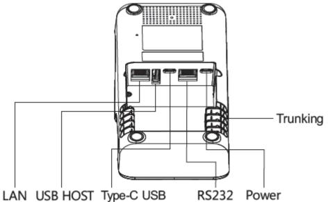
The matching diagram for A920Pro host and L920Pro wireless base is as follows:
