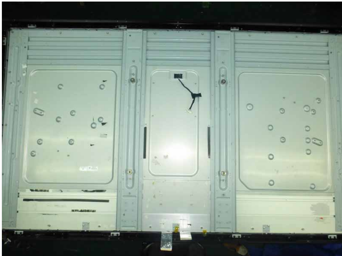
Figure 8 Backside of the LCD Panel
