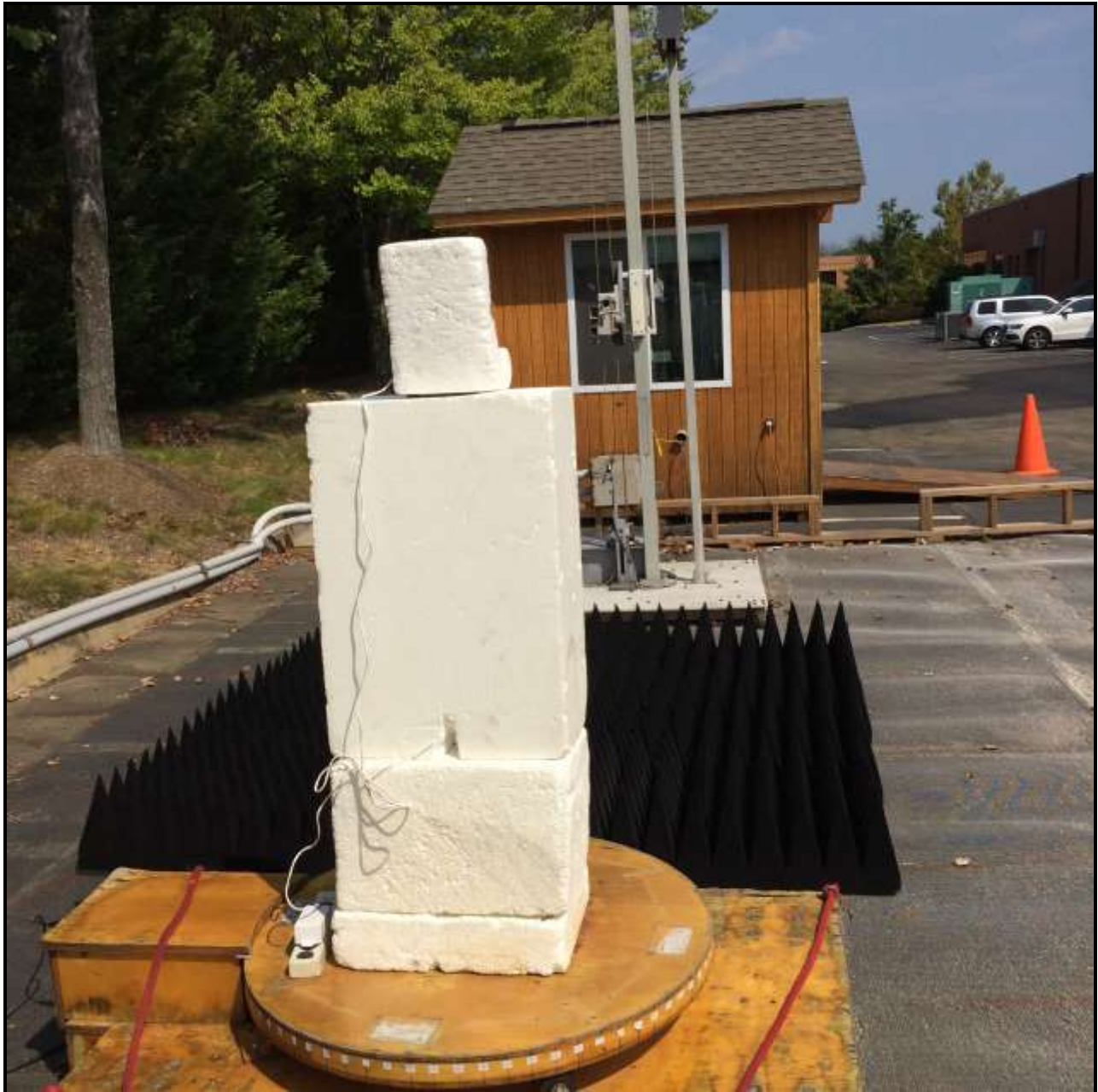
Photograph 2: Radiated Emissions Testing – Back View
