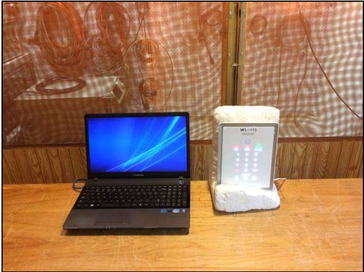
Photograph 3: AC Conducted Line Emissions Testing – Front View
