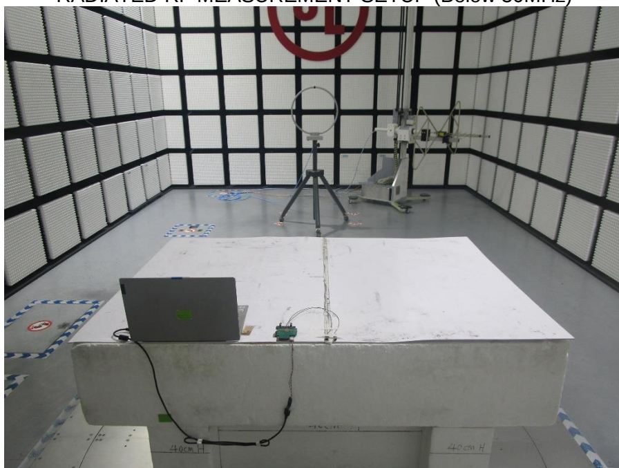
RADIATED RF MEASUREMENT SETUP (Below 30MHz)
