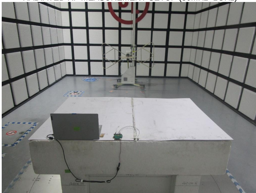
RADIATED RF MEASUREMENT SETUP (Below 30MHz)
