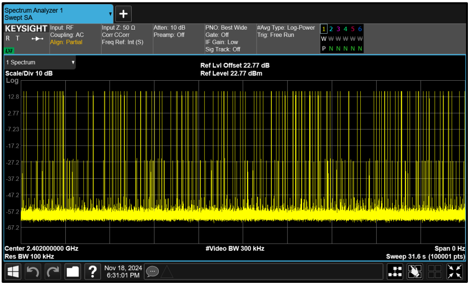
Figure 35 - 8-DPSK - 2402 MHz Accumulated Transmit Time
