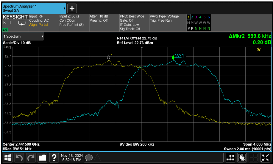
Figure 42 - \pi/4 DQPSK - 2441 MHz (CH39)
