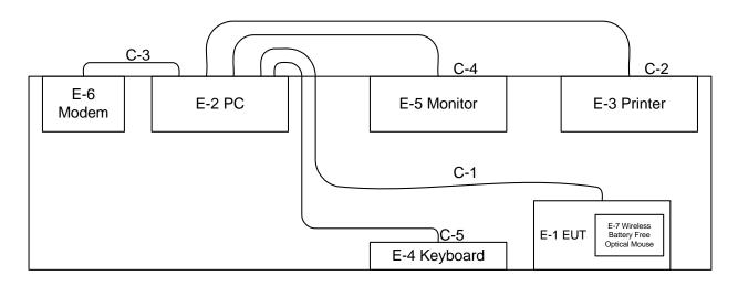
C-1 USB Cable C-2 Centronics Cable C-3 RS-232 Cable C-4 Video Cable C-5 Data Cable
