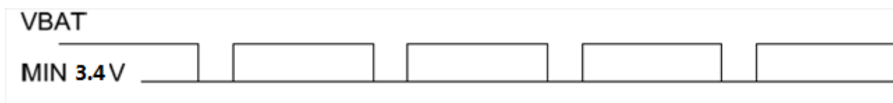
Figure4.4: VBAT lowest voltage drop
