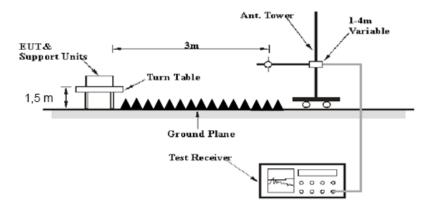
The radiated emission tests were performed in the 3 meters distance, using the setup accordance with the ANSI C63.10-2013. The specification used was the FCC 15.209, 15.247 and RSS-247 Clause 5.5, RSS-GEN Clause 8.10 limits.
