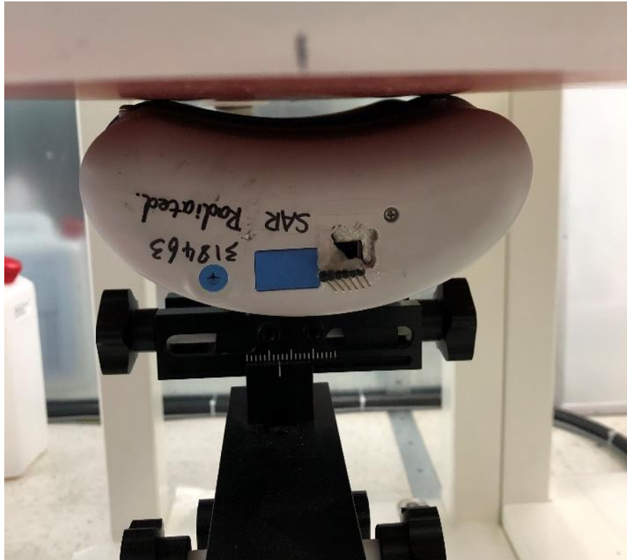
Top view of EUT against flat area of phantom with 0mm spacing Header added to allow control of BLE module.
