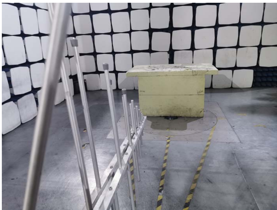
Radiation Emission Test Setup (30MHz to 1GHz)
