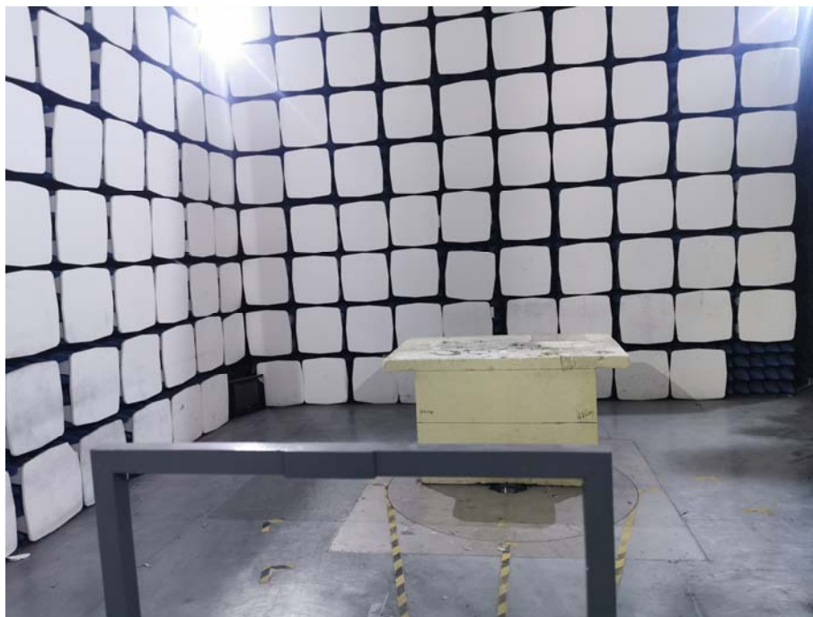
Radiation Emission Test Setup (Below 30MHz)
