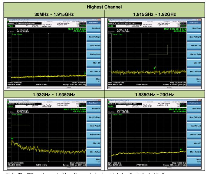
Note: The BS spurious out-of-band transmission level is below the indicated limit.
