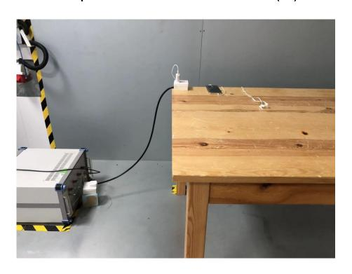
Set-up for Radiated Emission (RE), Below 1GHz
